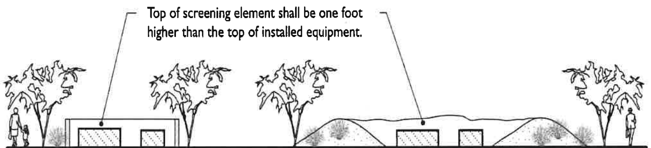
Figure 18.80.110.A.2. Screening of Ground-Mounted Equipment
